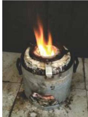
(b) In-house fabricated improved cookstove
